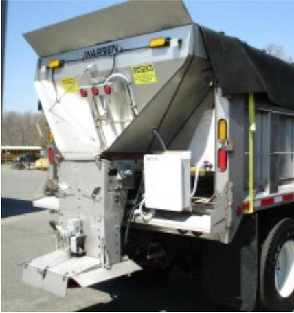
**The Warren Model AC-2420A** is a heavy duty hydraulically powered spreader designed to spread abrasives, chemicals, or mixtures of both for ice control, dust control, and abrasives for seal coating. Ideal for the operator looking for a long life economical unit rather than initial cost.
