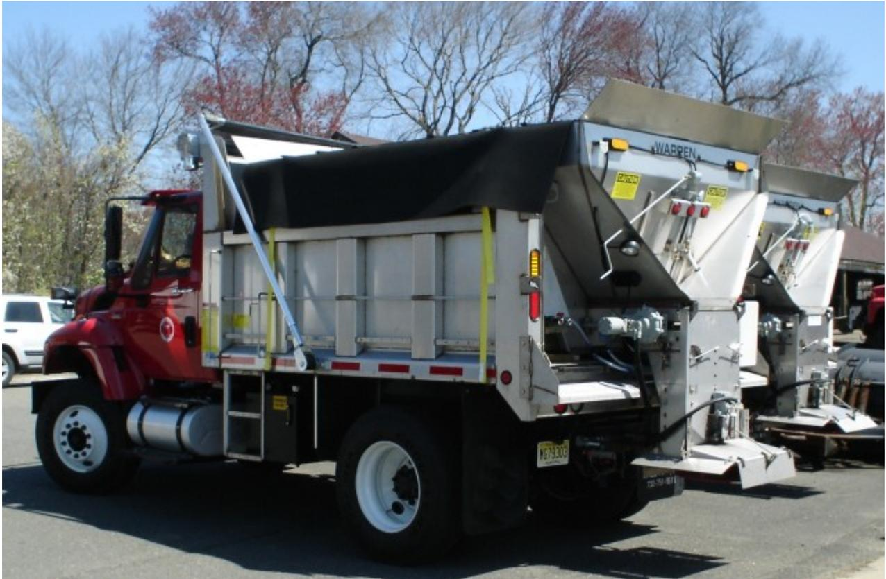
*The Warren Model AC-2420A can be either dump body or truck chassis mounted with a choice of either truck or auxiliary engine power. Heavy duty hydraulic components are mated to a heavy gauge ASTM-A1011-A45 high tensile steel hopper body (standard) for longer equipment life.*
